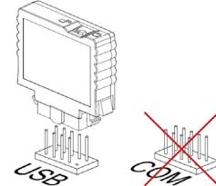
**note** It is easy to mix USB with COM port. Both have same or similar connector. Please read the motherboard user manual or the connector description on the motherboard to localize the USB port.
